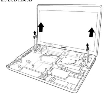
Figure 4-36 Removing LCD
